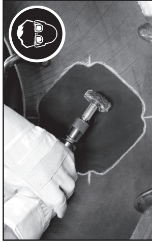
6. Use a smooth buffing tool to buff the liner inside the marked area. (Buffer should be max. 5000 rpm)
